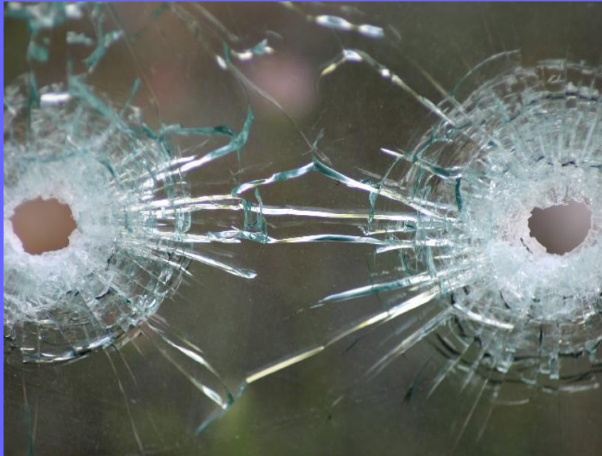
Radial and concentric fractures in a pane of glass.
