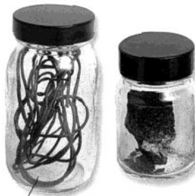
Glass evidence jars sealed with vapor barrier screw lids to contain volatile accelerants.
