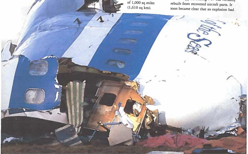
blown a hole in the fuselage. The blast wave tore the aircraft apart. The pattern of damage suggested that an explosion had occurred in cargo bay 14L. This explained a vital mystery: why had Flight 103 never sent a "mayday" signal? Bay 14L was adjacent to the plane's electricity supply, and the blast would have cut power to the radio. It also brought flight data and cockpit voice recording to an abrupt end, silencing the "black boxes."
